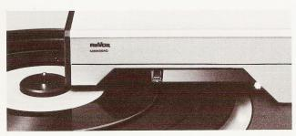
Press the button ◀ (inward) and keep it depressed until the tone arm has been transported over the record's run-in groove.
