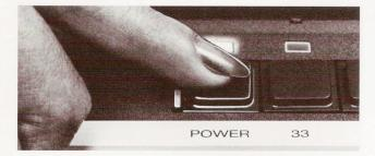
**Switching on**Press button POWER to switch the turntable on.
